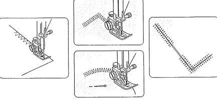
Here's How to Repair a Tear:
